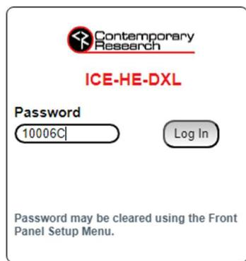
When the web page is first accessed, the browser will be directed to the login page. Enter the last six characters of the MAC address in the password field, then click the **Log In** button. The characters should be entered with no punctuation or spaces. Letters should be entered as upper case. i.e.: 10021A
