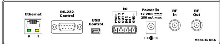
**Ethernet:** RJ-45 10/100 Ethernet connector for Web page access, Telnet, UDP control, and IPTV Streaming
