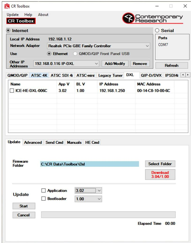
Check the box next to the ICE-HE-DXL in the list. In the bottom section of the CR Toolbox window, check the box next to **Application** and select the desired version from the drop-down menu. If also updating the bootloader, check the box next to **Bootloader** and select the desired version from the drop-down menu.
