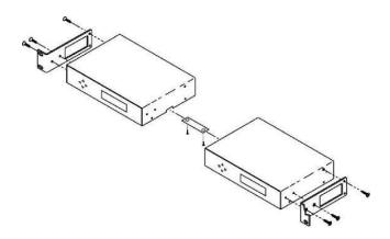
When mounting two components in one RU rack space, use the two short rack ears and the tie bar assembly.
