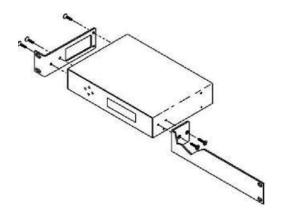
Attach a long and short rack ear to each side at the front of the unit, using five of the  $8-32 \times 1/4$ " screws.
