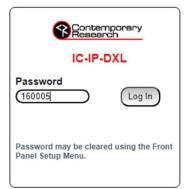
When the web page is first accessed, the browser will be directed to the login page. Enter the last six characters of the MAC address in the password field, then click the **Log In** button. The characters should be entered with no punctuation or spaces. Letters should be entered as upper case. i.e.: 16021A
