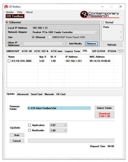
Check the box next to the IP-DXL in the list. In the bottom section of the CR Toolbox window, check the box next to **Application** and select the desired version from the drop-down menu. If also updating the bootloader, check the box next to **Bootloader** and select the desired version from the drop-down menu.
