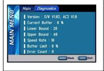
Displays decoder firmware and AC-3 software versions, current buffer usage, buffer parameters, and error count.
